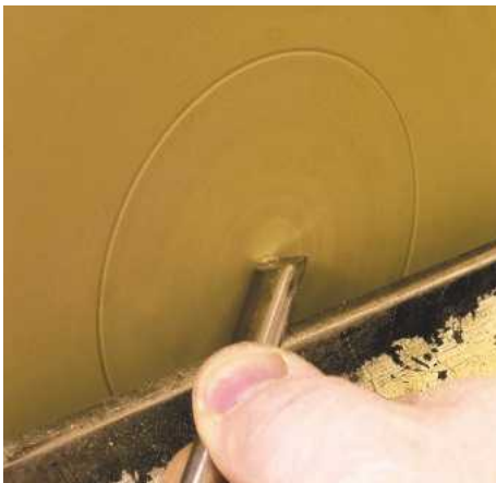
▲ Pic.4 Marking the centre of the foot with the point of a skew chisel will allow the bowl to be centred when it is remounted to remove the chucking point
